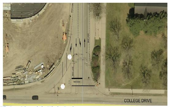
Figure 3 Bike Lane Schematic for Wiggins Road
